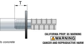
Threaded bars need to remain fully engaged and tight after installation and prior to concrete placement. Job site conditions may require additional inspection and/or re-tightening.
