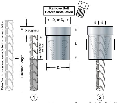
Cut bar to desired elevation - "X". Clean any debris and/or concrete off the deformed bar surface for the length that will be inserted into the T-Head. Grind down burrs and imperfections if necessary.
